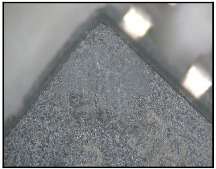
Marking (top-side) After mechanical resurfacing (Fail)
